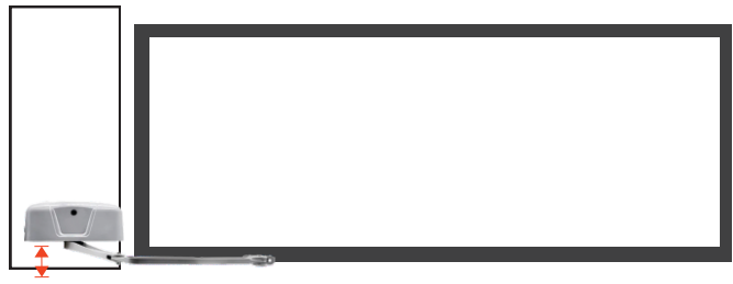
ABSOLUTE Minimum 40mm from ground to Gate Centre Rail
