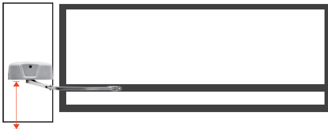
Ideal Minimum 90mm from ground to mounting Rail
